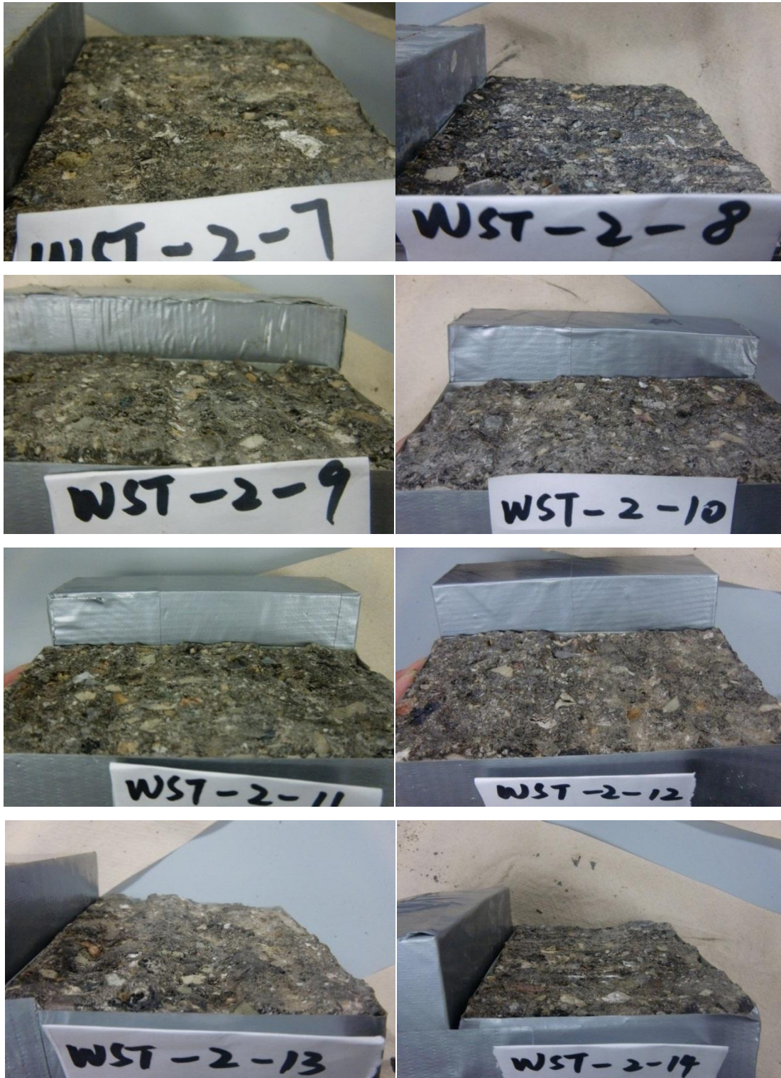
Figure 9 Conditions of the HMA surfaces for WST-2-07 to WST-2-14.
