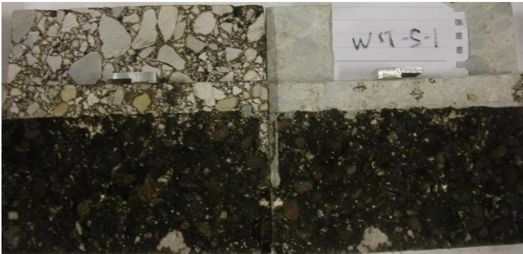
Figure 69 Failure surfaces of milled, dry and room-temperature specimen, WST-S-01.
