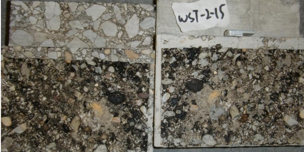
Figure 70 Failure surfaces of 45° milled, dry and room-temperature specimen, WST-2-15.
