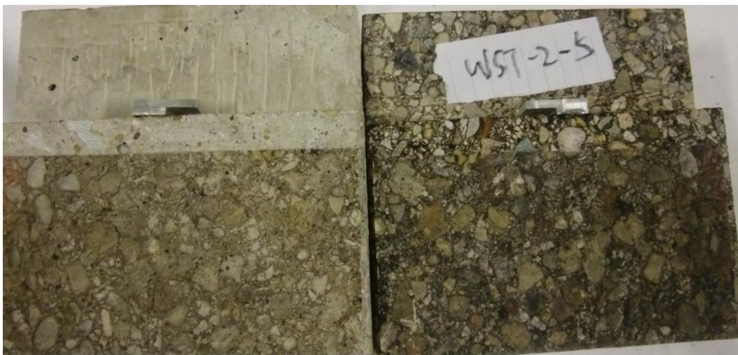
Figure 73 Failure surfaces of unmilled, dry and frozen specimen, WST-2-05.
